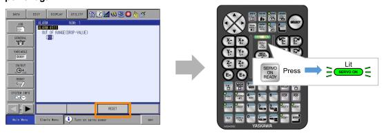
Press and hold [FWD] while the [SERVO ON] lamp is lit on the programming pendant.
