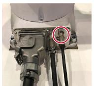
Connect the dummy connector for short-circuiting the safety signals to the SAFETY connector on the robot controller.
