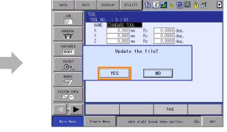
The measurement data will be registered in the tool file.
