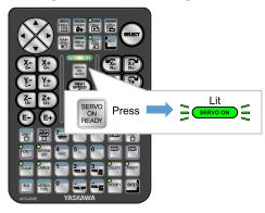
The [SERVO ON] lamp will be lit in green and the servo power will be turned ON.
