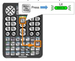
5. Press [SHIFT] and [TOOL SEL COORD] to display the TOOL NO. SELECT window, and place the cursor on the tool number to change.
