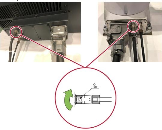
4. Use the same procedure to connect the torque sensor cable to the [TQ] connector on the manipulator and the [-X73] connector on the robot controller.
