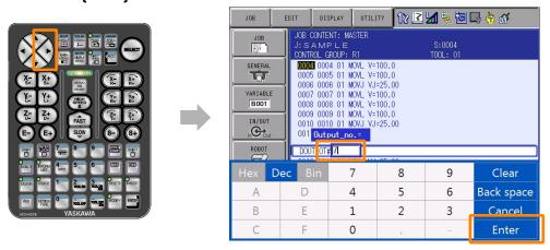
5. Move the cursor to "ON" with the cursor keys on the programming pendant, and press [SELECT] to toggle ON/OFF.
