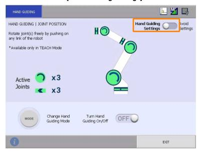
6. Press (MODE) until the manipulator operation mode changes to the mode to select.
