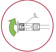
Use the same procedure to connect the torque sensor cable to the [TQ] connector on the manipulator and the [-X73] connector on the robot controller.
