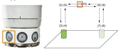
If the arm speed feels fast, tap (double-click) the [MOVE] button twice, and then move the arm when all three buttons are flashing. The arm will move slowly, and it will be easier to make fine adjustments because the feeling of arm coasting will be reduced.
