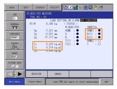
12. While squeezing the enable switch on the back of the programming pendant with the left hand, press and hold [FWD] until the manipulator stops.
