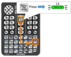
Information If the movement speed seems slow or fast, press MANUAL SPEED [FAST] or [SLOW] to change the speed at which the manipulator moves.
