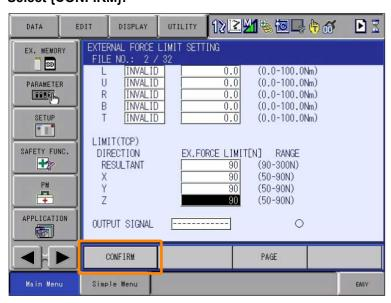
{FILE SET STATUS} will change from "CONFIRMING" to "COMPLETED", and the setting will be applied to the CPU in the robot controller.
