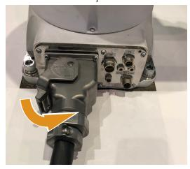
2. Use the same procedure to connect the X1 connector on the manipulator cable to the robot controller.
