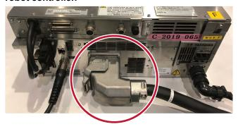
Connect the switch/lamp cable to the [SW] connector on the manipulator and the [-X74] connector on the robot controller.
