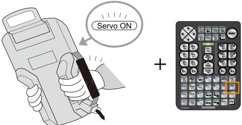
While [FWD] is pressed and held, the manipulator will move to reference position 1 to start
