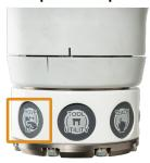
12. While the [MOVE] button on the manipulator is pressed, manually move the arm of the manipulator to the location to be taught.
