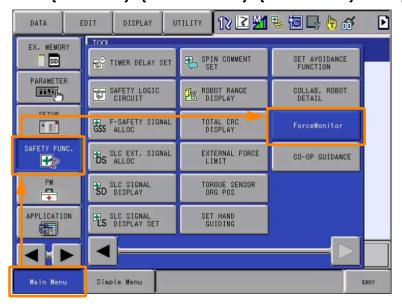
2. Select {External Force}, and check the torque values by external force of each axis.
