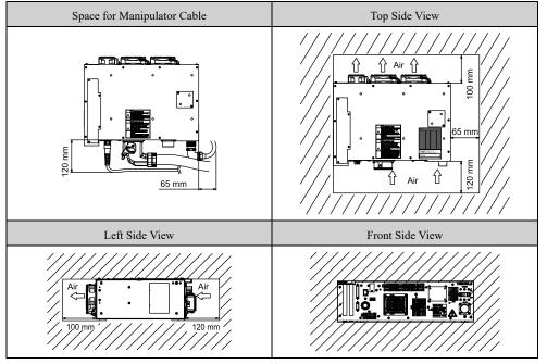
2. Ensure the following space when the YRC1000micro robot controller is side mounted.
