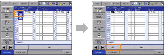
5. Confirm that there are no mistakes in the safety logic circuit, and then select {CONFIRM} and {YES}.
