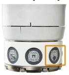
The position of the manipulator will be registered as step 2 when the [TEACH] button is pressed.
