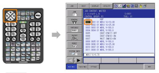
Information If the tool number column is not displayed, touch {DISPLAY} - {ENABLE TOOL NO}.
