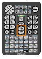
Information Selecting medium speed at first is recommended to make it easier to check the movement of the manipulator.
