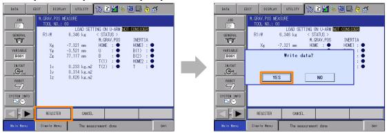
The measurement results will be written to the robot controller.
