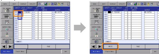
Confirm that there are no mistakes in the safety logic circuit, and then select {CON-FIRM) and {YES}.
