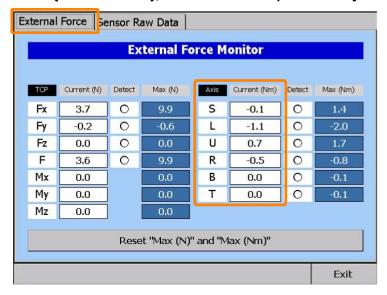
3. Compare the current values to the values when the manipulator first started being used and check if the difference between the values is growing larger.
