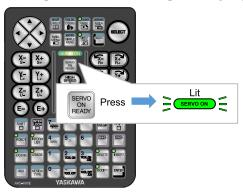
The [SERVO ON] lamp will be lit in green and the servo power will be turned ON.
