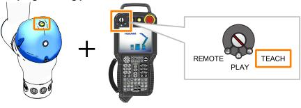
If the LED is not lit, the collaborative operation function is disabled. Refer to the following section and enable the collaborative operation function.
