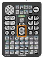
Information Selecting medium speed at first is recommended to make it easier to check the movement of the manipulator.
