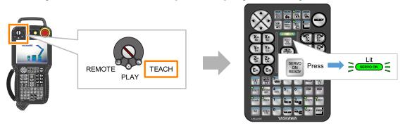
7. If "ALARM 4511 OUT OF RANGE(DROP-VALUE)" is displayed, first press {RESET}, and then press [SERVO ON READY] on the programming pendant to turn ON the servo power again.
