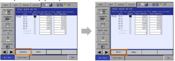
A confirmation window will be displayed when transferring and saving the configured data to the robot controller is completed.
