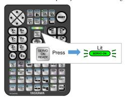
While squeezing the enable switch on the back of the programming pendant with the left hand (the [SERVO ON] lamp is lit on the programming pendant), press and hold [FWD] until the manipulator stops.
