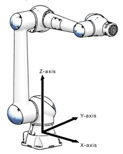
• Relationship between Programming Pendant Axis Keys and Manipulator Movement
