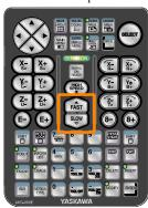
4. Move the cursor to step 10 by pressing the cursor keys on the programming pendant.
