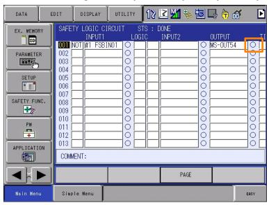
The following table gives the details of the MS-OUT54 output signal.
