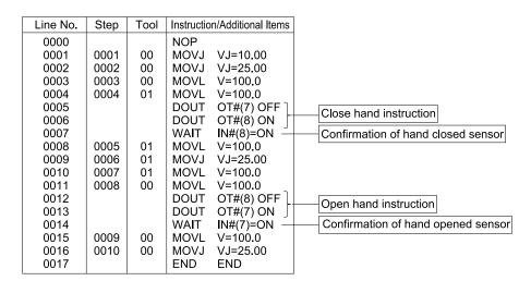
This program uses the tool shown below. The following four signals must be connected to open and close this tool.
