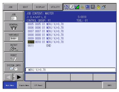
Information The speed of manipulator motion, opening and closing the hand, the tool files, and other settings are configured after this procedure. This procedure registers the positions of the manipulator only.
