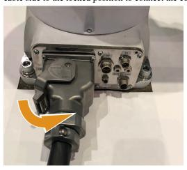
Connecting the Robot Controller
