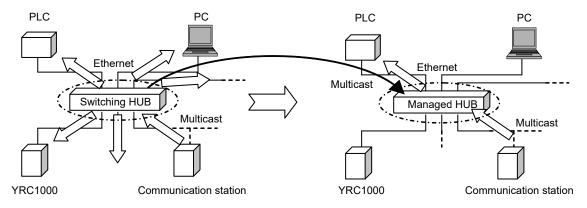
Use of the Switching HUB transmits the packets to all devices
