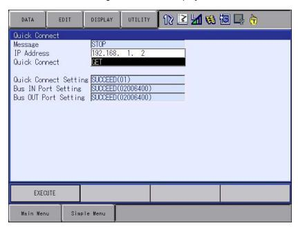
If the QuickConnect setting information is as following, the QuickConnect setting is valid, and the setting after step 8 is unnecessary.
