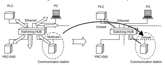
Broadcast/multicast transmits the packets to all devices.
