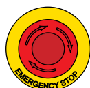
Fig A: Emergency Stop Button
