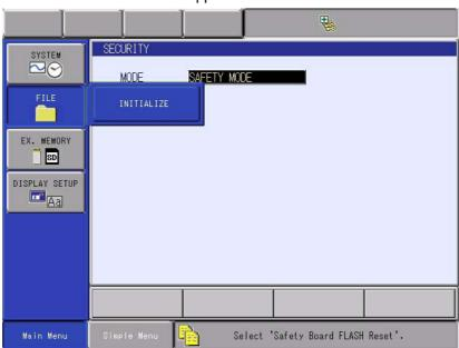
7. Move the cursor and select "Safety Board FLASH Reset" on the window.
