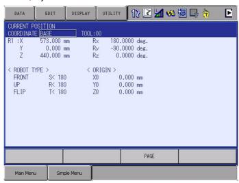
7. Set the recorded Rx, Ry and Rz values to {REF. ANGLE} on the tool angle monitoring condition file window.
