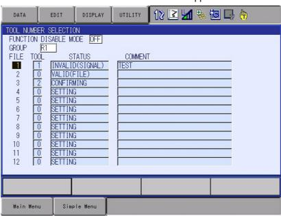
On the status list window, the sixteen setting files for the tool number selection function are arranged so that their status can be confirmed. By scrolling down the window, all the list can be seen.
