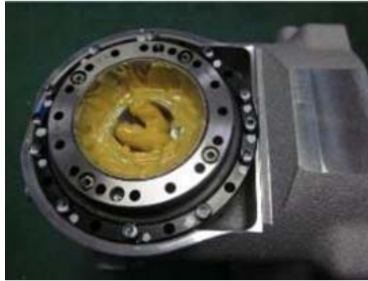
Fig. 6-7: Example of B-Axis Grease Application (Flex Spline)
