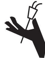
If the wire is projected from the end tip of the welding torch, it may poke you in the eyes or face.
