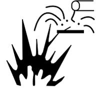
Spatters or hot base metal immediately after welding may result in fire.
