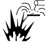
Spatter and metal powder inside the welder may cause a deterioration of insulation resulting in accidental fire.
