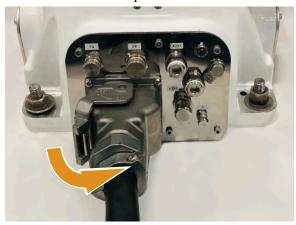
2. Use the same procedure to connect the X1 connector on the manipulator cable to the robot controller.
