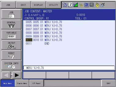
Information The motion and speed of the manipulator, opening and closing the hand, the tool files, and other settings are configured after this procedure. This procedure registers the positions of the manipulator only.
