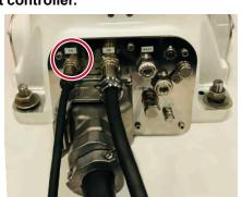
Connect the dummy connector for short-circuiting the safety signals to the SAFETY connector on the robot controller.
