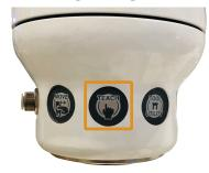
The position of the manipulator will be registered as step 2 when the [TEACH] button is pressed.
