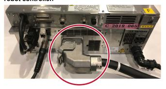
3. Connect the switch/lamp cable to the [SW] connector on the manipulator and the [-X74] connector on the robot controller.
