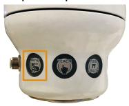
12. While the [MOVE] button on the manipulator is pressed, manually move the arm of the manipulator to the location to be taught.
