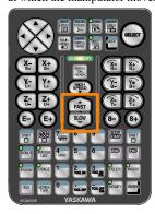
4. Move the cursor to step 10 by pressing the cursor keys on the programming pendant.
