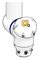
Information If the LED is not lit, the collaborative operation function is disabled. Refer to the following section and enable the collaborative operation function.
