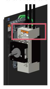
Close the robot controller door and turn the door lock 90 degrees counterclockwise.
