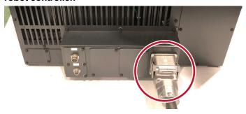
3. Connect the switch/lamp cable to the [SW] connector on the manipulator and the [-X74] connector on the robot controller.
