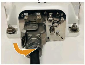
Use the same procedure to connect the X1 connector on the manipulator cable to the robot controller.
