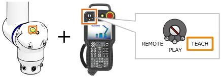
Information If the LED is not lit, the collaborative operation function is disabled. Refer to the following section and enable the collaborative operation function.
