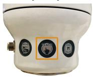
The position of the manipulator will be registered as step 1 when the [TEACH] button is pressed.
