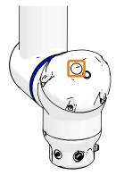
If the collaborative operation LED is lit, the collaborative operation function is enabled. Refer to the following section for the operating procedure to disable the function.
