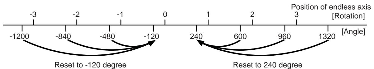
Perform teaching so that the rotation starts at a position between 0 to 360 degree when you want to rotate the axis in "+" direction or so that the rotation starts at a position between -360 to 0 degree when you want to rotate the axis in "-" direction.
