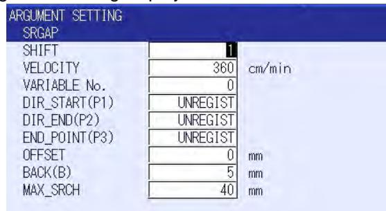
5. Move the manipulator to the travel start point (P1), and press [MODIFY] with the cursor on "UNREGIST" of P1, then press [ENTER] to register the position of P1.
