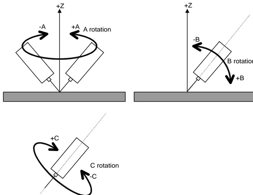
A: Rotates around the Z-axis in the base coordinate system
