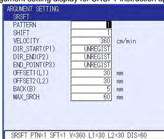
5. Move the manipulator to the travel start point (P1), and press [MODIFY] with the cursor on "UNREGIST" of P1, then press [ENTER] to register the position of P1.
