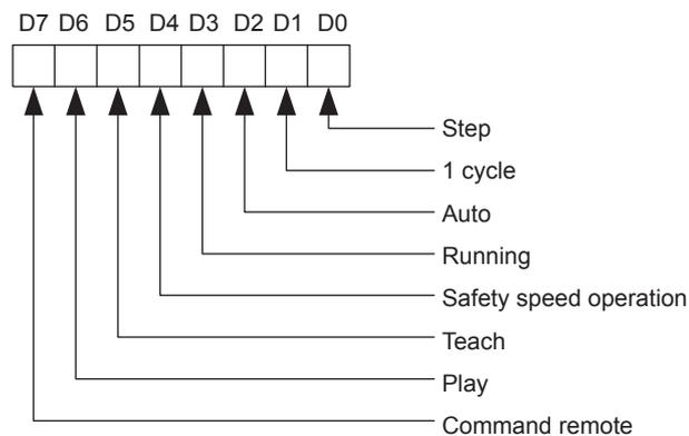
Data-2 = Represented by the following bit data coded into a decimal number
