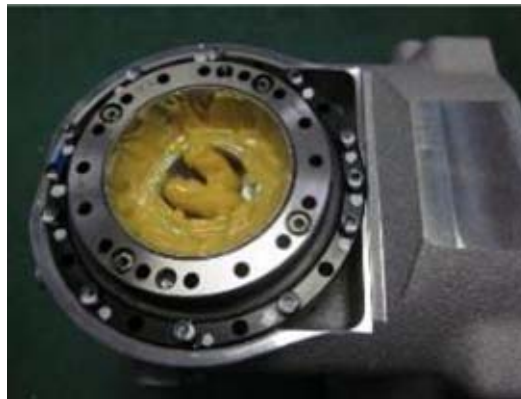
Fig. 6-8: Example of B-Axis Grease Application (Flex Spline)
