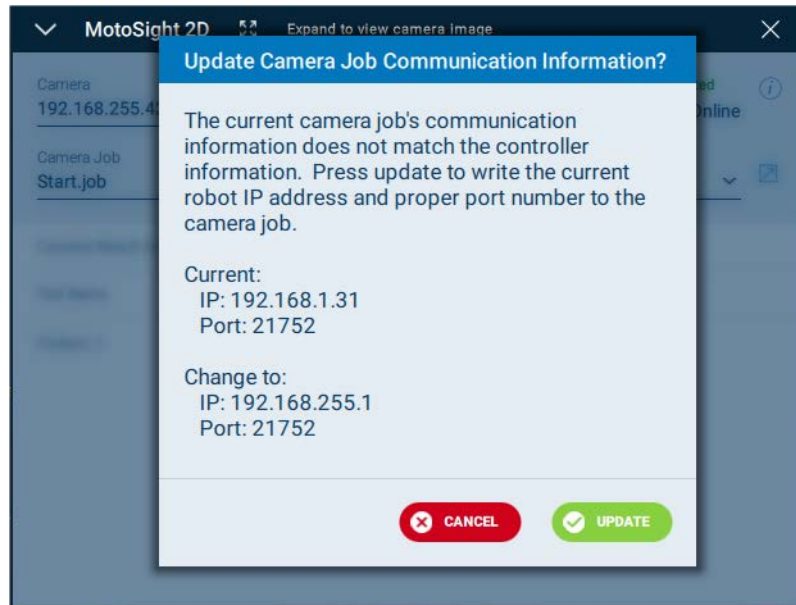
Fig. 2-11: Updating Camera Job Communication
