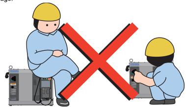
Do not let unauthorized personnel touch the Robot Controller or the pendant while power is ON.
